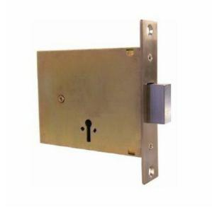
Mortice dead lock for FB1 or FB2 Fire Brigade key Case width 110mm, height 78mm, thickness 15mm Backset 52mm Forend size 118mm x 22mm Supplied with flat strike plate and all fixing screws FB1 Mortice lock - FB1M FB2 Mortice lock - FB2M
